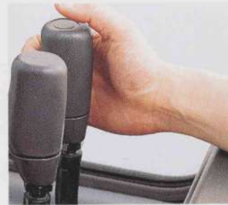
Servo-assisted two-lever hydraulic control, with "kickdown".
