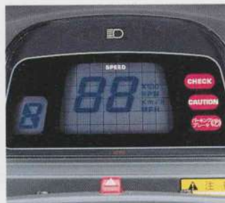
Main monitor for information also on driving speed and gear engaged.
