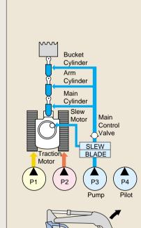
■VARIABLE DISPLACEMENT, AXIAL PISTON, HYDRAULIC PUMPS WITH POWER SHIFT enable system flows and pressures to vary according to the load placed on the hydraulic system. The hydraulic system puts to work all of the available engine horsepower for maximum operating efficiency.
